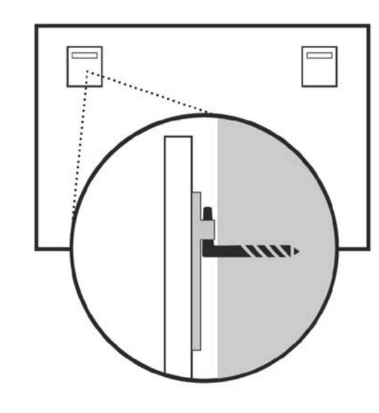
3 Each wall mounting must be hung on the appropriate hooks.
