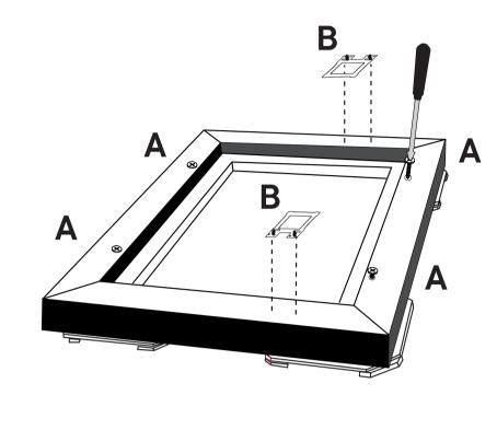
3 Now screw the floater frame and the mounting hooks onto the photo canvas using the supplied screws.
