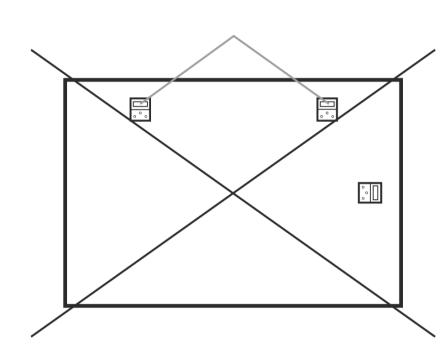
2 Hang the product on the designated mount. The mounting device is pre-assembled. Please do not attach a piece of string or wire to the wall mountings and hang this over a single hook in the middle!
